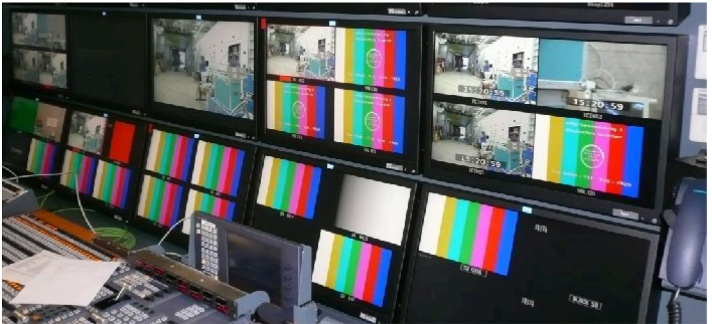
Customized Monitor Wall in an OB truck built with BLACK MILAN QLM 124W and SPARROWHAWK LSM 124W HD
