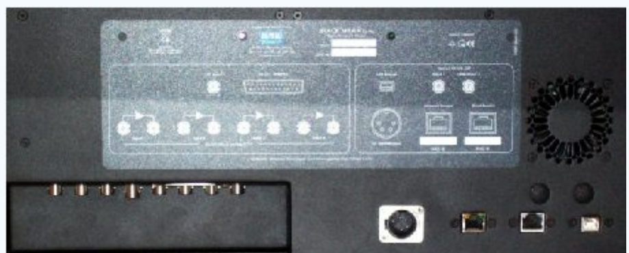
Four universal SD/HD-SDI Inputs with loops and analog CCVS capability. Two TCP/IP ports for MultiViewer and Monitor remote in the BLACK MILAN series
